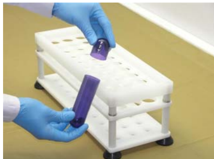
1. Separate the caps and bodies of capsules. Keep the caps in a bowl.
