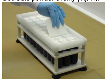
6. Spread any extra powder. Repeat tapping till all the powder is filled in the bodies. Typically, after 3-4 tapping cycles no more powder will enter bodies.
