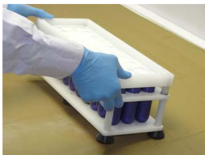
5. While holding the top sheet and body sheet together lift the filler from one side by 1 cm (1/2 inch) and then drop it back on the table. Repeat for each of the four sides (one tapping cycle). See Tip B .
