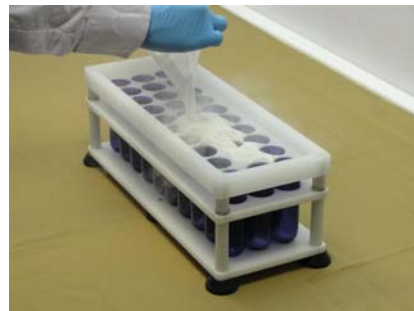
3. Pour pre-measured powder on to the Filler. When pouring, distribute powder evenly ( Tip A ).
