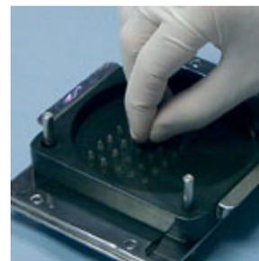
9. Place the top caps of the capsules back onto the bottoms, pressing to fully lock each capsule.
