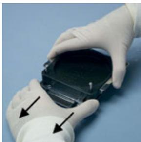
7. Slowly pull out the Spacer Plates one at a time. Hold Capsule Holder with both Handles as you pull out each Spacer Plate and then gently let it down.
