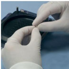
3. Separate capsules one at a time and place caps in a shallow container such as a Petri dish.
