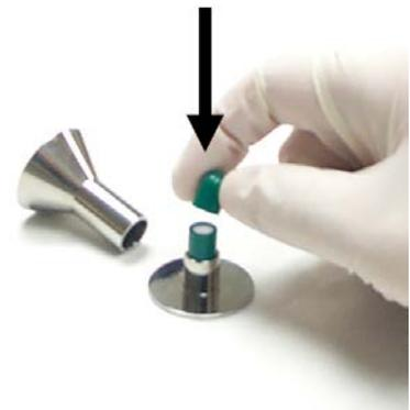
**6.** Place the capsule's cap onto the body of the capsule, pressing firmly to lock. Remove the filled capsule from the base.
