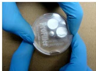
5. Rotate the top disc 90° clockwise to close cavity in middle disk.
