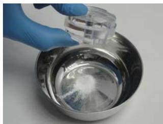
6. Turn over Tap DensiMeter and tap out any remaining powder in the top disc.
