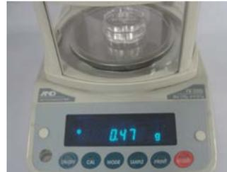
7. Weigh filled Tap DensiMeter. Your tapped density is the final weight. Example 0.47g means a tapped density of 0.47g/ml.
