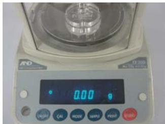
1. Place empty Tap DensiMeter on balance and tare the balance.
