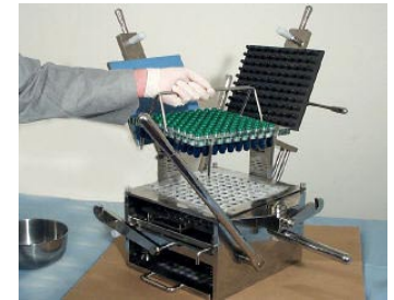
16.) Remove the capsule tray and you now have filled, locked capsules ready for packaging!
