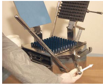
6.) Push the cam handle away from you to drop the bodies so they are even with the top sheet.
