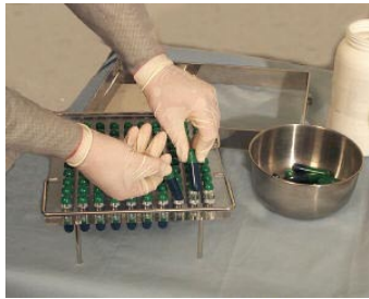
1.) Load capsules into the tray.
