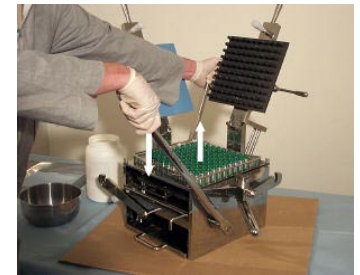
4.) Hold rear handle and push down on the locking lever to separate the capsules.
