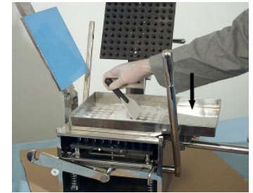
8.) Pour & spread the pre-measured powder. Move extra powder onto the powder reservoir.
