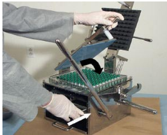
13.) Push the sliding frame in and lower the locking plate.
