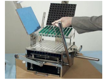
12.) Return the tray containing the caps to the Filler.
