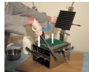
4.) Hold rear handle and push down on the locking lever to separate the capsules.
