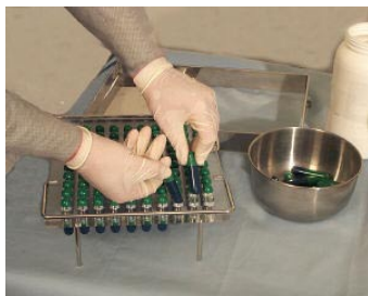
1.) Load capsules into the tray.
