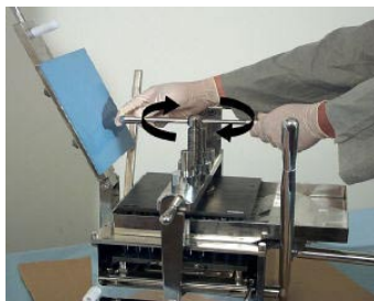
10.) Turn the tamping plate screw handle to compress the powder. This allows you to fill more powder in each capsule.
