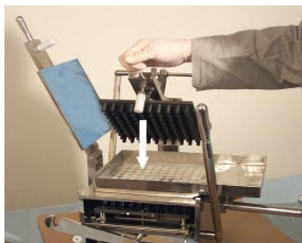
9.) Lower the tamper and lock it using the "C" clamp.
