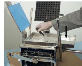
8.) Pour & spread the pre-measured powder. Move extra powder onto the powder reservoir.
