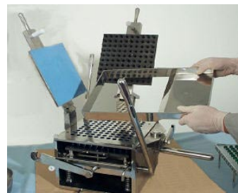
7.) Place the powder tray onto the Filler. The tray will keep powder from spilling.
