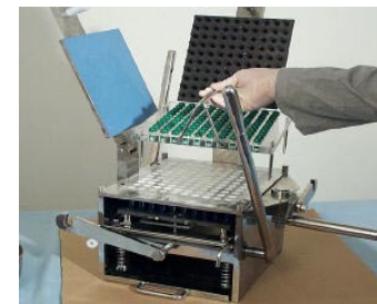
12.) Return the tray containing the caps to the Filler.
