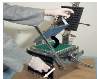
15.) Lift the locking plate and pull the sliding frame out to set for next batch of capsules.
