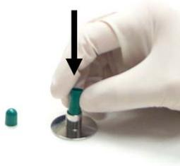
1. Separate a single capsule. Place the capsule body (longer, narrower part of the capsule) in the Holder. See note below
