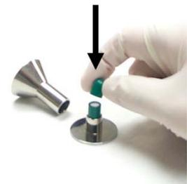
6. Place the capsule's cap onto the body of the capsule, pressing firmly to lock. Remove the filled capsule from the Holder.
