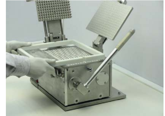
9. Remove Powder Tray and spread remaining powder. When using Vibrator, there may be a small amount of powder under the Powder Tray. Spread the powder into capsules. To reduce this effect, use Powder Tray with Clamps. See Accessories.
